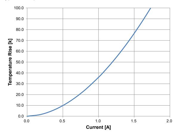
**Typical Temperature Rise vs. Current Characteristics**
